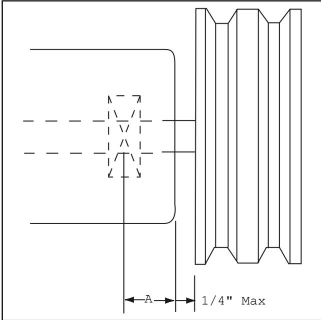
$$\text{*Belt Pull lbs} = \frac{275000 \cdot \text{Motor HP}}{\text{Blower RPM} \cdot \text{Sheave Diameter}}$$
